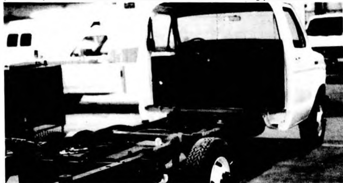
Cab and chassis of a 1991 Ford E350 cutaway van with 7.31 diesel motor is the starting place for the custom built ambulance.
