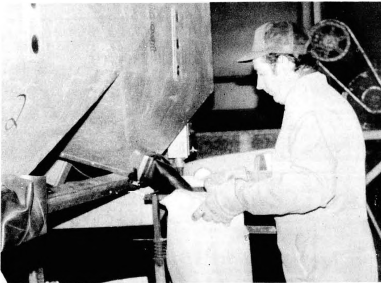
Ed Bruneau filling bags of rice as it comes out of the length grader.
