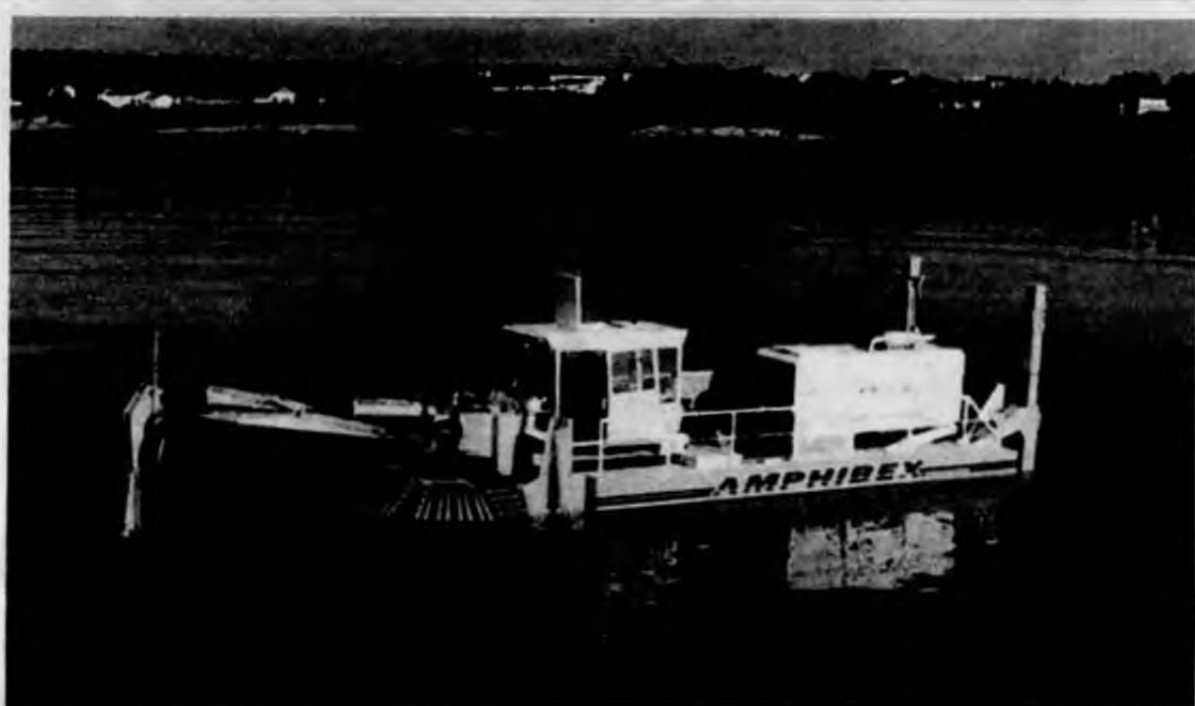
An Amphibex ice-breaking machine converted to a dredge.
